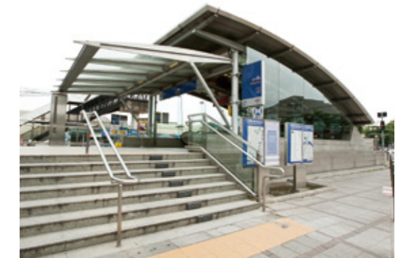
The entrance to the Bang Sue station of the MRT Blue Line. As a flood prevention measure, the station entrance is elevated from the road.
