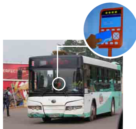
Bus fares can be paid by tapping a contactless smart card against an orange terminal next to the driver.
