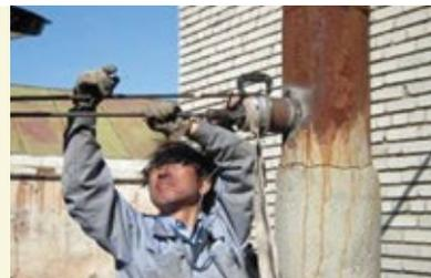
Performing on-site stack gas measurement
