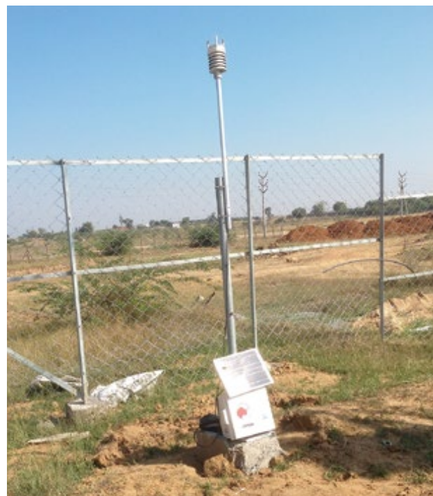
An Automatic Weather Station (AWS) set up under the research project Information Network for Natural Disaster Mitigation and Recovery in India.
