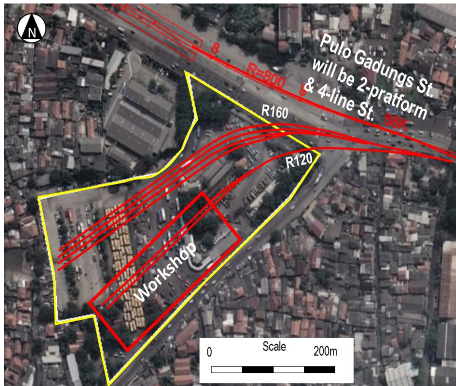
E8 : Workshop, Stabling & Inspection Tracks
