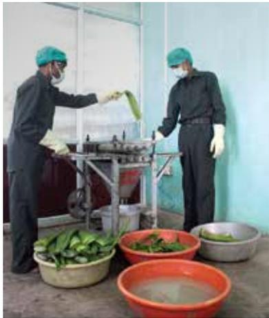
▶ Aloe Vera gel is extracted from a crushing machine.
