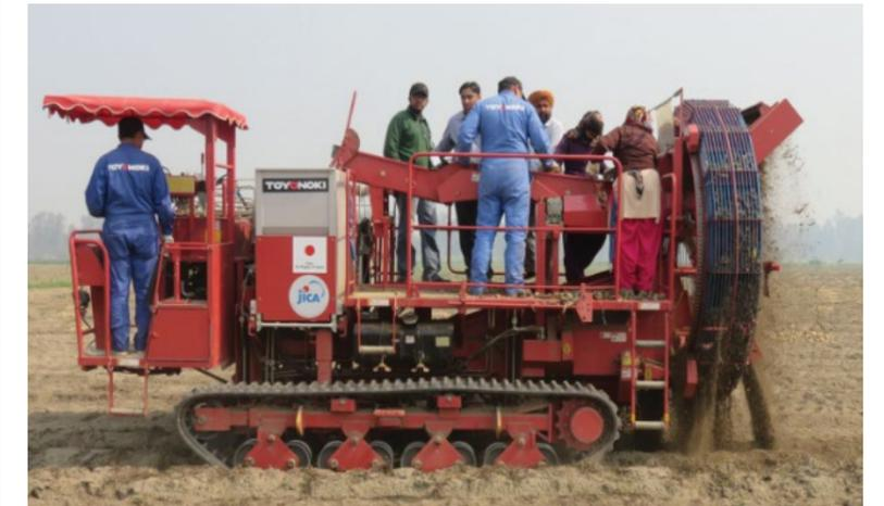
Introduction of **Self-propelled Potato Harvester** in Punjab that demonstrated efficacy for **enhancement of yield rate** and **reducing of damage rate to less than 5%, the standard** which could be contributing to productivity improvement.
