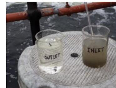
Comparison of inlet (raw sewerage, right) and outlet (treated water, left) at Okhla STP
