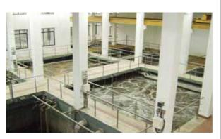
The MBR system ensures space saving. Automatic control and centralized monitoring for water and sewage treatment processes are carried out through PLC and SCADA. The BNR process is applied for denitrification and dephosphorization.
