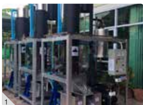
1. Small ice machine with 3 ton/day ice making capacity 2. Installing Cold Room 3. Completed Cold Room 4. Pickup Truck for cold chain
