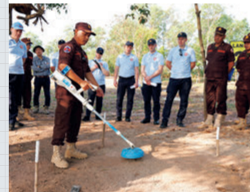
Practical training on the use of ALIS, the Advanced Landmine Imaging System developed by Professor SATO Motoyuki of Tohoku University.
