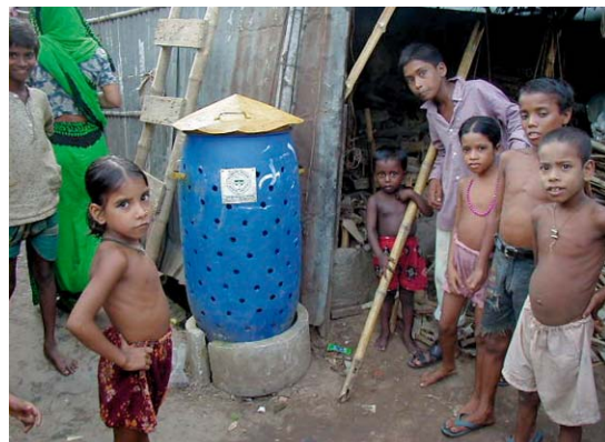
Photo 2-1 An example of equipment used to produce compost from food residues in a slum.
