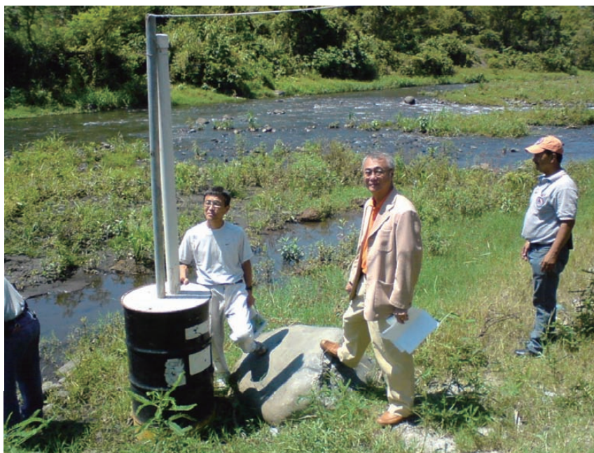
Figure 9: Water Glass (Water Level Monitor) with Automatic Warning System in Guatemala
