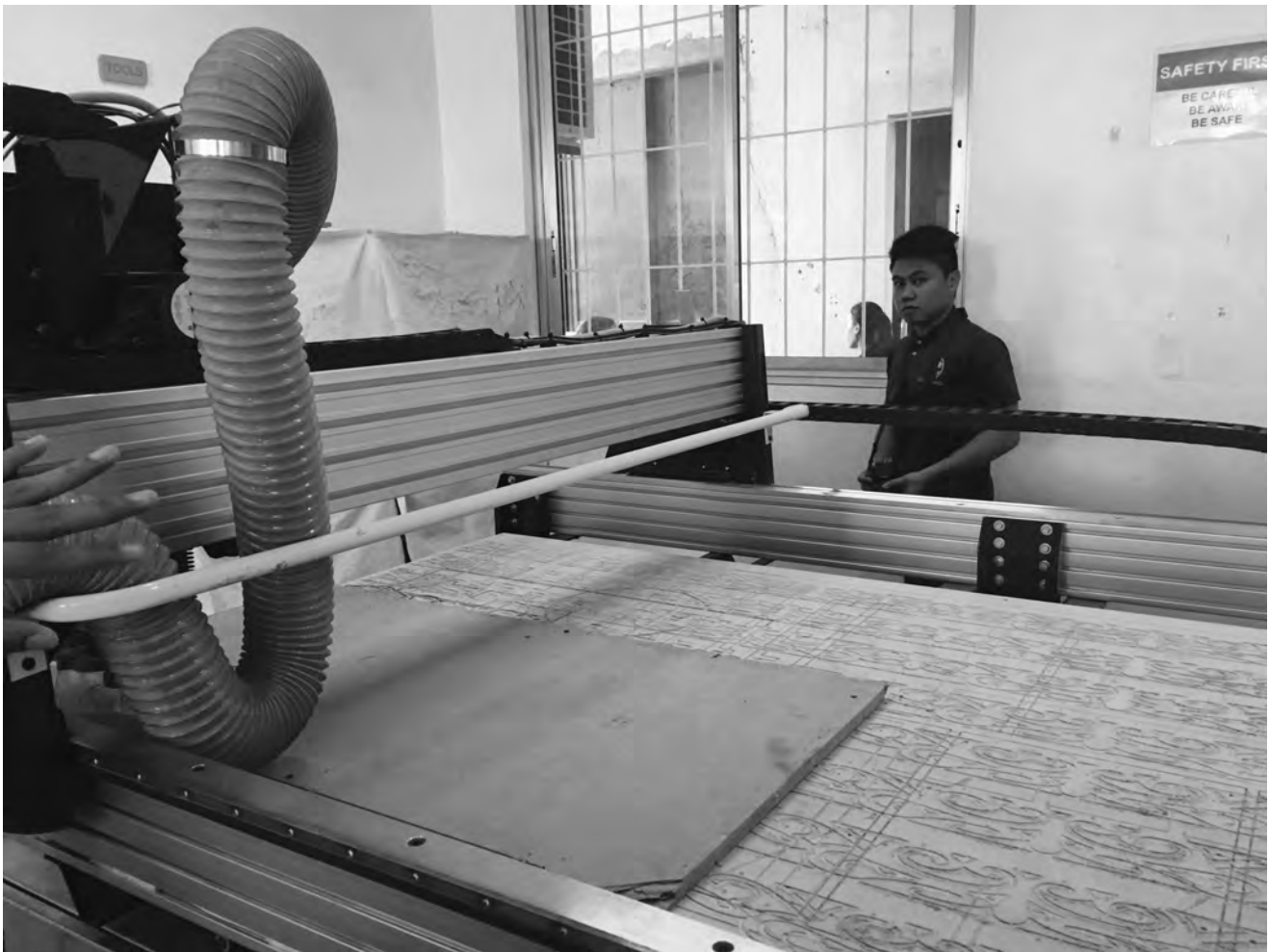
Figure 2.3. A Fab Lab Bohol employee demonstrates the large computer numerically controlled (CNC) milling machine, which cuts designs into 3-D
