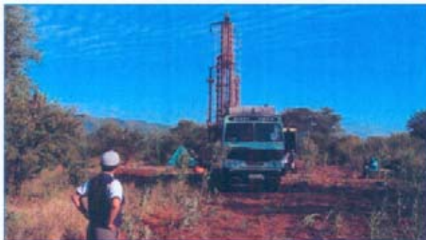
Test drilling in one of the target areas.
