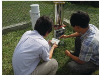
Monitoring of rainfall on site (by rain gauge)
