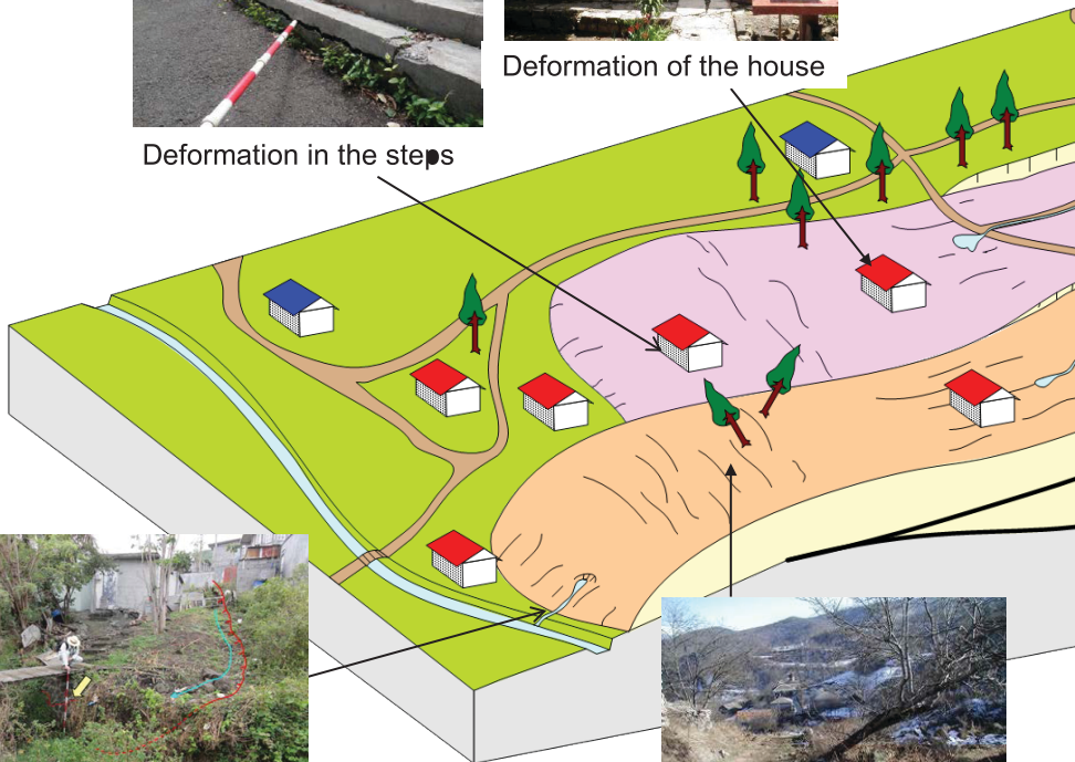
Deformation of the toe of landslide block
