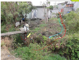
Deformation of the toe of landslide block
