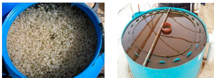
Photo.2 Biofilter and Sedimentation tank
