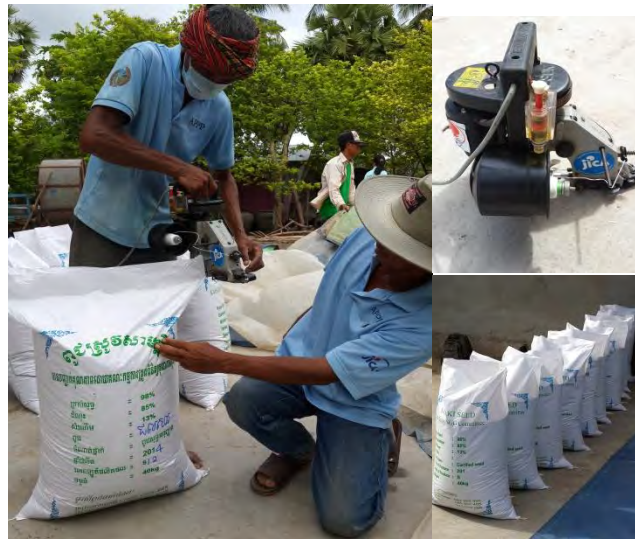
④ Seal the shipping bag by sewing machine. Write seed information by marker.
