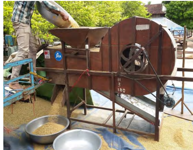
② Remove unfilled paddy by winnowing. Adjust the winnower to get only fulfilled paddy.
