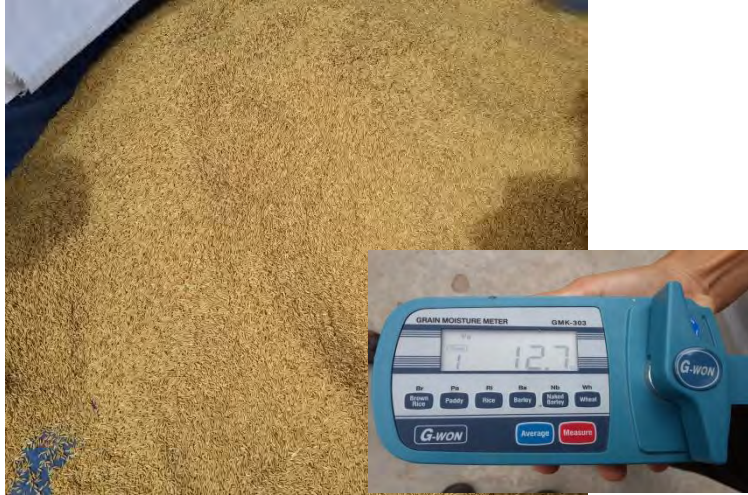
① Check the moisture content of the paddy before starting winnowing.
