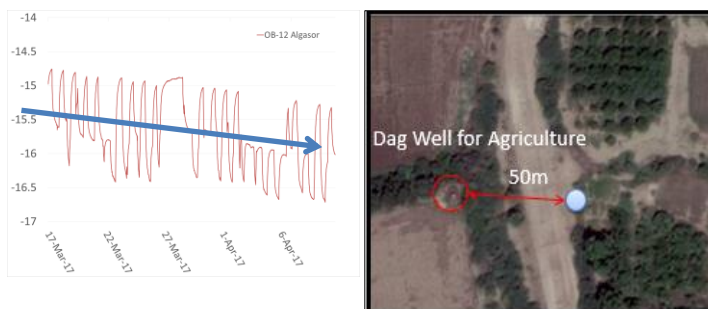
Figure 3-3. Record of water level of an observation well which is affected by irrigation well
