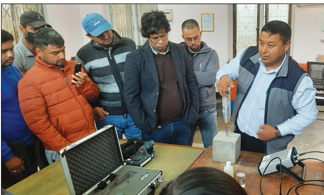
Using of Schmidt Hammer in Lab
