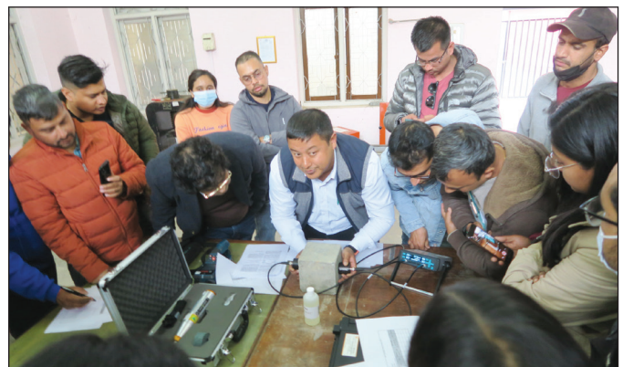
Using of Ultrasonic Pulse Velocity Tester in Lab
