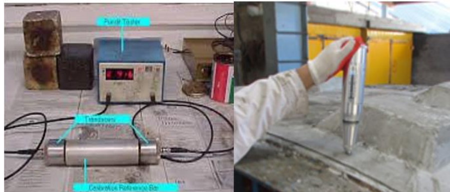
Figure 2: Ultrasonic Pulse Velocity Meter & Schmidt Hammer
