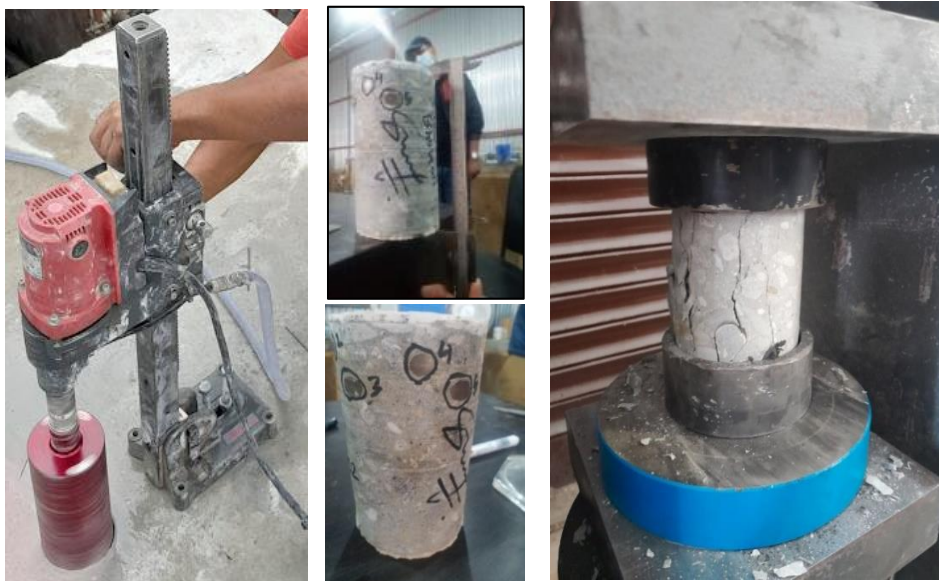
Figure 2: Core cutting, measurement & testing
