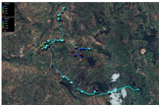
Photo 1: Example of a Pipe Network Model and Hydraulic Calculation (Rwamagana District)
