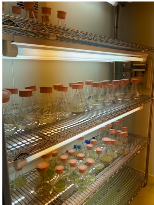
Figure 1. Duckweed culture in a growth chamber with regulated temperature, humidity, and a light-dark cycle.
