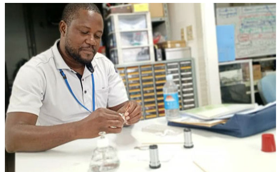
Mr. Simusiko servicing lenses for the slight lamp an ophthalmic equipment used for diagnosing, treatment and management of various eye conditions or diseases
