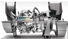
30 MW class gas turbine Source : Kawasaki Heavy Industry
