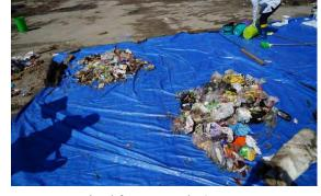
Conical quartering (over 30 kg of waste was remained for segregation)
