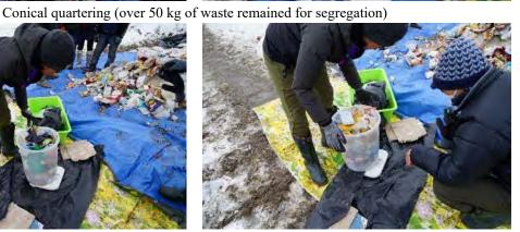
Measurement of bulk density of waste
