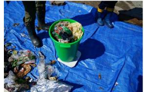
Measurement of bulk density of waste
