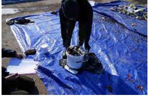
Measurement of bulk density of waste
