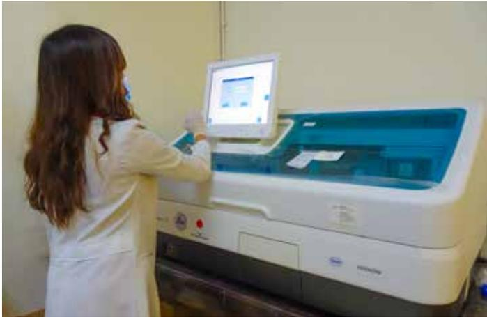
**CAPTION** The cobas e 411 analyzer provided to San Lazaro Hospital is a fully automated analyzer that has high sensitivity, reliability, and reproducibility of results which uses ElectroChemiluminescence (ECL) technology for immunoassay analysis that can be used for a broad range of applications including infectious diseases.
