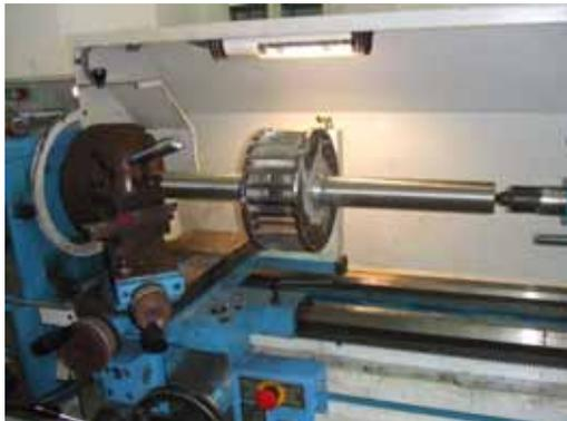
Crossflow turbines designed by CeMTRE
