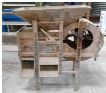
Figure 11: Hand-operators wooden-framed mechanical winnower.
