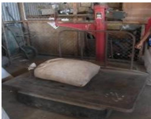
**Figure 18: Platform type of weighing scale.**
