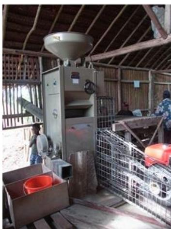
**Figure 13: Impro: PS-80 (a copy of Satake SB10D).**
