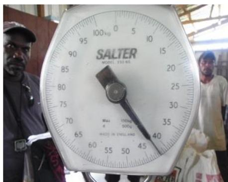
**Figure 20: Hanging type of scale 100Kg capacity.**
