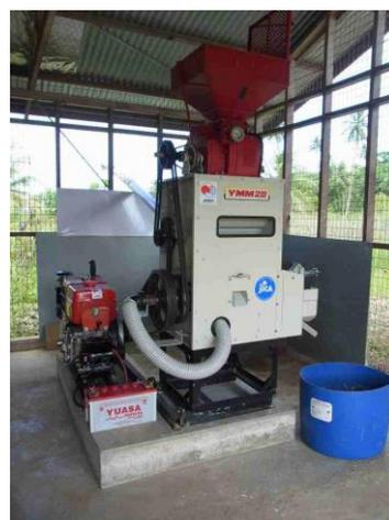
**Figure 14: Yanmar YMM20 milling unit.**
