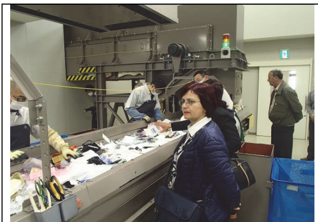
Ogaki Recycle Center. Here, recyclables collected from households are sorted by materials manually. Then, the recyclables are packed by a compressor.
