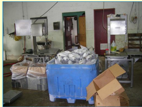
Frozen fish cut into steak by band saw
