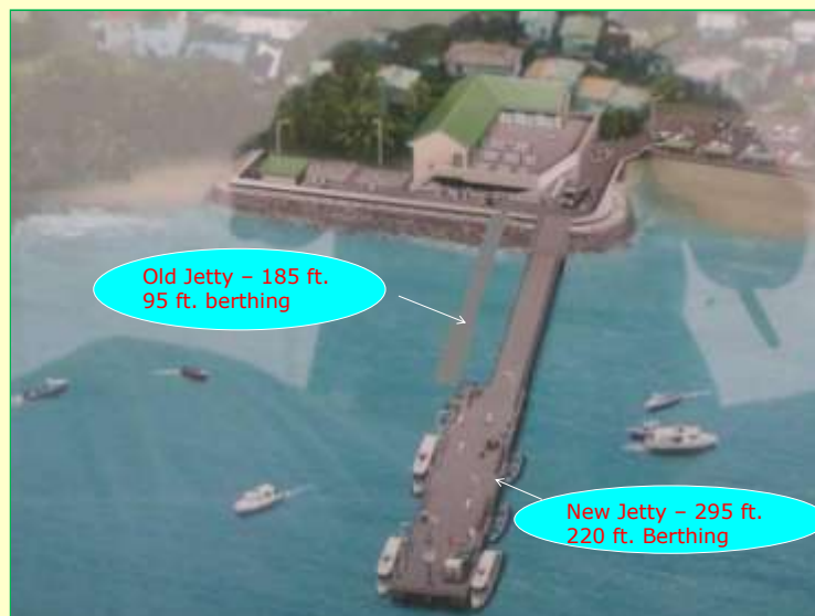
Bird view image of existing old jetty and new jetty under construction
