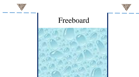
Figure 4-5: Examples of Freeboard
