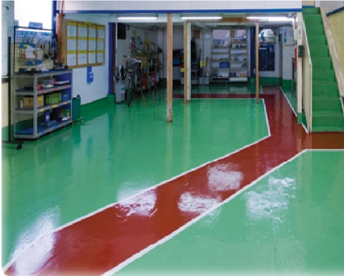
Fig.3 The walking way and the working area are separated to avoid traffic and for employee safety
