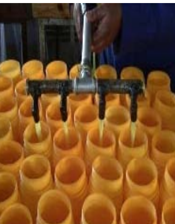
Elimination of Muda of motion and transportation by introducing filling hose saves labor force & increase productivity.
