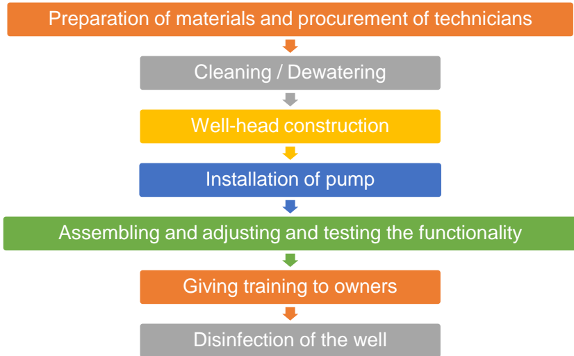
Figure 5: Steps of rope pump installation
