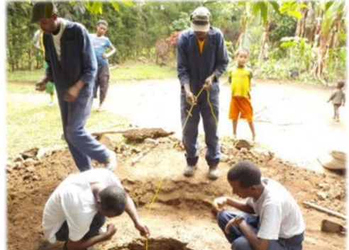
2. Measuring depth and static water level of well and checking well condition
