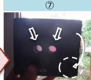
Turn color disk, and see holes. Turn color disk until finding out same color(Right and Left). This result shows "Free Chlorine" [mg/L].
