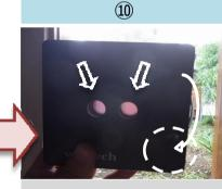
Turn color disk, and see holes. Turn color disk until finding out same color(Right and Left). This result shows "Total Chlorine" [mg/L].
