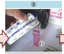
Add one "DPD No.3" into sample cell(1). And then, crash and mix it using the crash rod. This is for "Total Chlorine" check.
