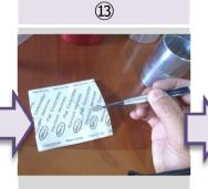
Prepare membreme filter(0.45µm), open the firm cover, and take filter using sterilized forceps.
