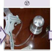
Vacuum sample water using hand pump.
