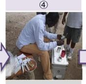
Sterilize all filtering tools, sampling cup using ignited alcohol.
