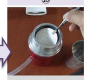
After getting pass sample water to filter, pick up the filter carefully using forceps.
