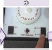
Select temperature switch to 44 degreeC, and turn on "ON".
