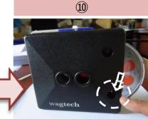
Read number in hole. This is concentration of Fluoride [mg/L]. If "0.5" is shown, result is 0.5 mg/L as Fluoride.
