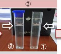
Add 10 mL sample water into 2 sample cells until upper line.
