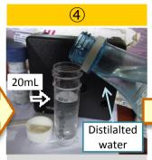
Add distillated weter into 20mL tube until 20mL line.
