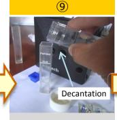
Decant sample water into sample cell until 10mL.
