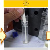
Crash and wait 10 minutes. And then, set sample cells into comparator with color disk for Nitrate[NO<sub>3</sub>]
