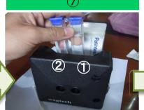
After that, set sample cells into comparator.
