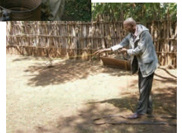
Baseline Survey: measuring depth of the well (Dale, January 2014)
