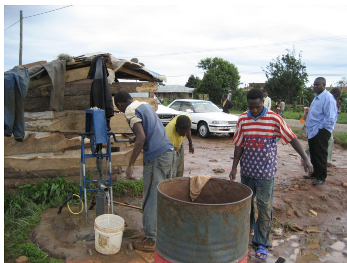
At a car washing, they are using water lifted by rope pump
