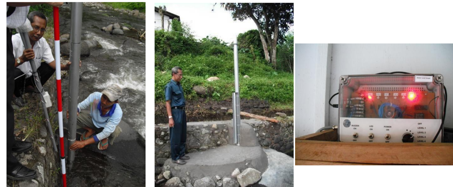
Rain Gauge Installation and Training for Observation to local people (Kali Jompo, Kab. Jember : Feb- Mar, 2010)
