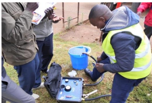
Meter accuracy test using calibrated bucket and portable meter tester (Ruiru-Juja WSP)
