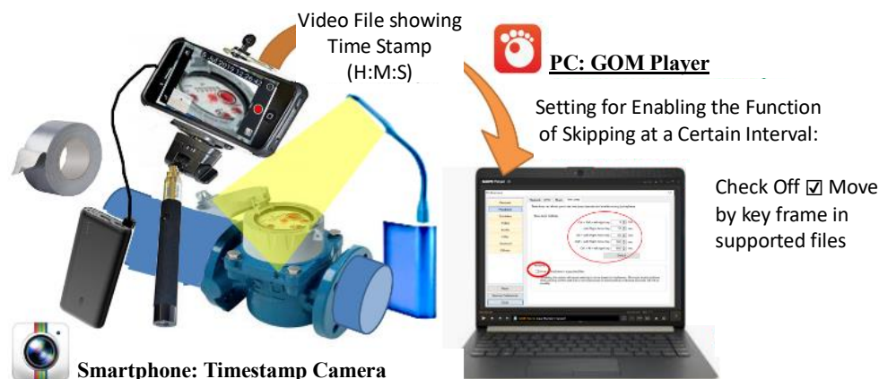
Figure 6. Measurement of the hourly fluctuation of water distribution with low-cost smartphone & free software (Trial)
