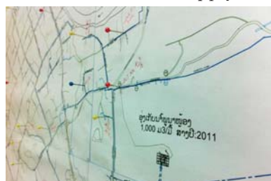
Leakage (repair) points marked by dress pin on a map
