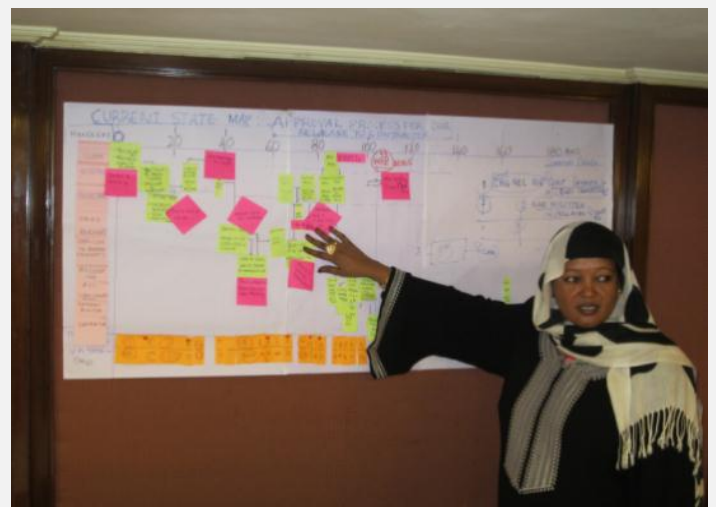
Process Mapping: It is a method which visualizes the workflow by putting the person in charge along the vertical line and the time along the horizontal line. Indicate the process by yellow and emphasize Muda (strain) by red tags.
