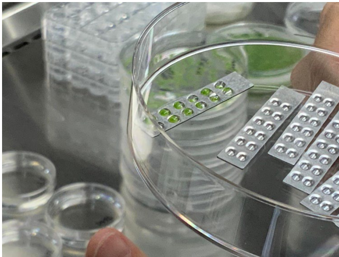
Figure 4: Cryopreservation on a small aluminum plate.
