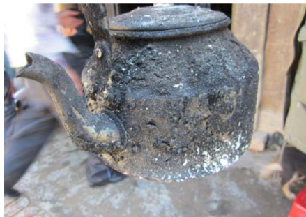
Kettle with 2.5 mm soot attached
