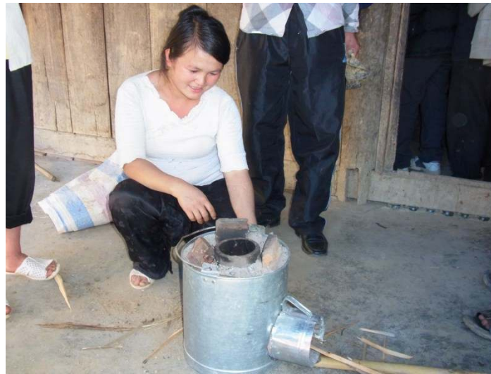
Portable-type rocket stove
