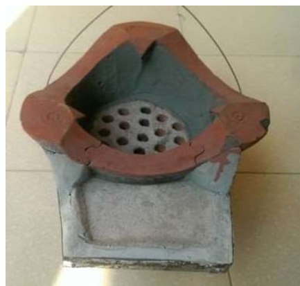
Photo 6: Traditional Lao stove Fuelwood are placed on the top.
