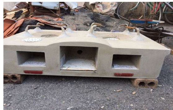
Photo 12: ICS available in Muong Gion commune (made in Quynh Nhai center). It is made of cement and has a large hole in the middle for an electric fan to provide air to two pans. There are two drawers under the hole.
